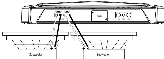
**To power one sub**, connect the positive wire from the single subwoofer to the left + terminal, and the negative wire from the subwoofer to the right - terminal.
