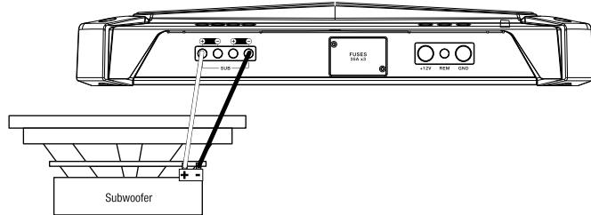
**NOTE:** Minimum speaker impedance for subwoofer operation is 2 ohms.
