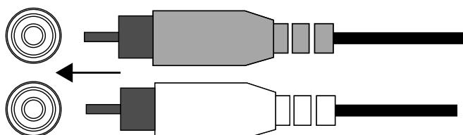
**If your car audio system's head unit does not have line-level outputs,** use the supplied bare wire-to-RCA adapters to connect the Stadium amplifier's inputs to either the front or the rear speaker outputs of your car audio system's head unit (splice crimps not included).
