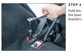
Fold the rear seat down, remove the nut at the base of the seat belt bracket, and slide the bracket off of the stud.
