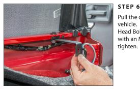
Pull the carpet down from the side of the vehicle. Slide a Rear Bracket over the Flange Head Bolt, under the rail, as shown. Secure with an M8 1.25 Hex Flange Lock Nut, and hand tighten. Repeat for the second hole.
