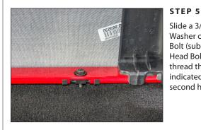
Slide a 3/8 " Flat Washer and a 3/8" Nylon Washer over an M8 x 30 mm 1.25 Flange Head Bolt (substitute an M8 x 45 mm 1.25 Flange Head Bolt for vehicles with hard top), and thread the assembly through one of the holes indicated in the previous step. Repeat for the second hole.
