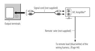
\* Firmly connect the ground wire of the amplifier to the car's chassis to avoid damaging the unit.
