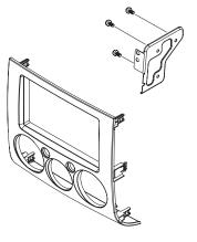
NOTE: REAR SUPPORTING THE STEREO ADDS TO THE INSTALLATION'S STRUCTURAL INTEGRITY. REAR SUPPORT AVAILABLE SEPARATELY.
