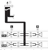
Perform these connections when using a subwoofer without the optional amplifier.
