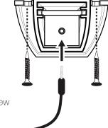
Remote cable passes audio; do not run cable parallel to power wires.
