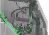
LPHTSL01 (B) Located in the right rear side of the trunk under the trim panel. This is the factory amplifier location and is attached to the OEM subwoofer enclosure.
