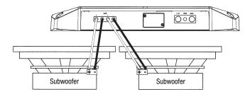
**To power one sub,** connect the positive wire from the single subwoofer to the left + terminal, and the negative wire from the subwoofer to the right - terminal.
