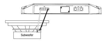
**NOTE:** Minimum speaker impedance for subwoofer operation is 2 ohms.
