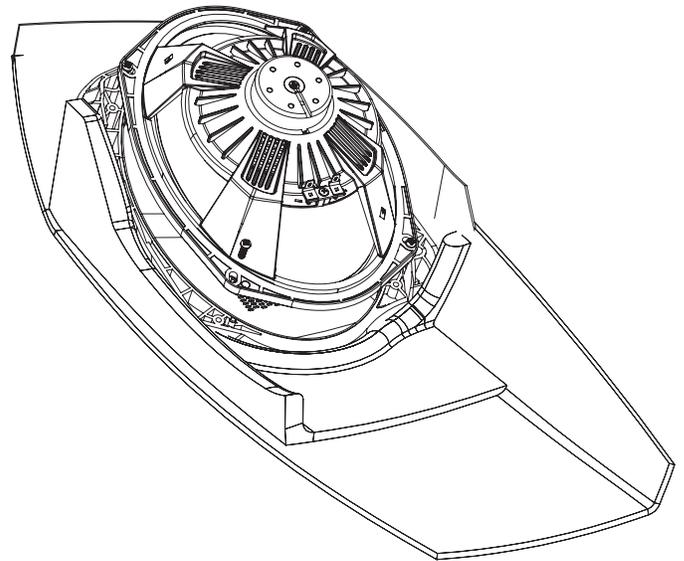
Step 6. Next you will attach the speaker, grille and mounting ring to the lid using the supplied screws.
