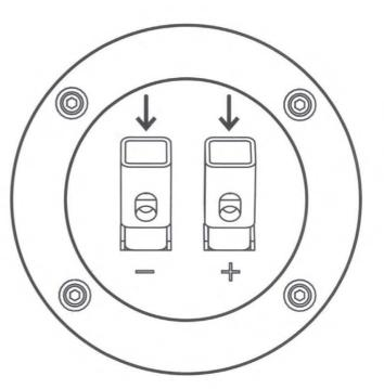
Plug your subwoofer speaker wire into the terminals using the red connector as positive and the black connector as negative. Connect the other end of the wire to your subwoofer amplifier in accordance with its owner's manual.
