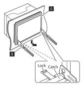
When the lower level is removed, remove from the upper two catches of the trim plate (6).
