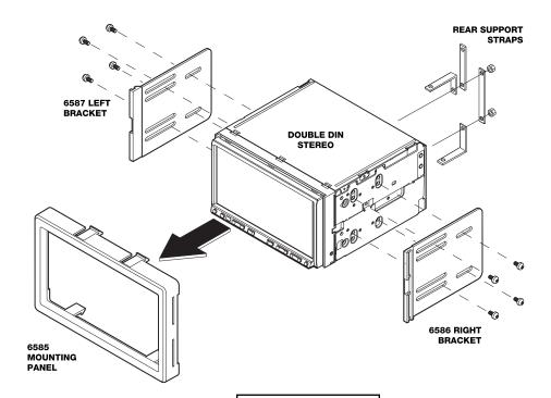
NOTE: REAR SUPPORT AVAILABLE SEPARATELY. REAR SUPPORTING THE STEREO ADDS TO THE INSTALLATION'S STRUCTURAL INTEGRITY.
