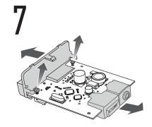
Remove plastic ends and screws from PCB board.
