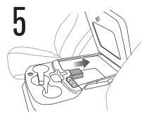
Disconnect the plugs then depress the 4 locking tabs (2 on top and 2 on the bottom) and push the module forward to release it.
