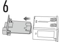
Release locking tabs and pull the board out.
