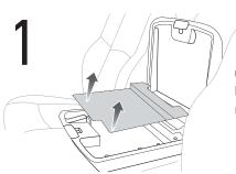
Open the center console lid and remove the rubber matt.
