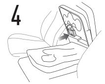
Push tabs and push the module forward to release it
