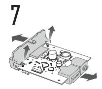
Remove plastic ends and screws from PCB board.
