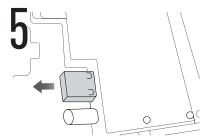
Disconnect the plugs then depress the 4 locking tabs (2 on top and 2 on the bottom) and push the module forward to release it.
