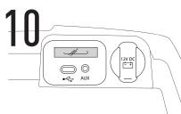
Reassemble the center console. Mask the SD slot with the sticker provided.
