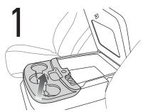
Open the center console lid and remove the cup holder cover.
